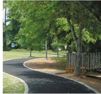
Rubberized Asphalt Concrete (RAC) trail surface
