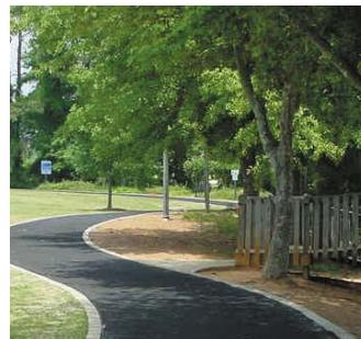
*Rubberized Asphalt Concrete (RAC) trail surface*
